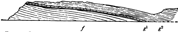
FIG. 12.—SECTION ON THE NORTH BANK OF THE RIVER ONNY AT CHENEY LONGVILLE FOOTBRIDGE, SHROPSHIRE; SHOWING THE PENTAMERUS-BEDS LYING UNCONFORMABLY ON THE OLDER STRATA.— f . W. Salter.
